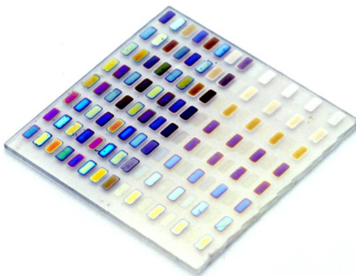
Figure 3. The 128-member binary library prior to sintering. The dimension of each sample is 1 \times 2 \text{ mm}^2 . The colour of each is the natural colour of light reflected from a white-light source (reproduced from [7]).
